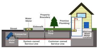
An example of a water service line. The utility owned portion spans from the water main connector to the property line or a curb-stop. The customer-owned portion is the part of the service line that extends from the curb-stop to the meter box or isolation valve in the building's premise plumbing.
